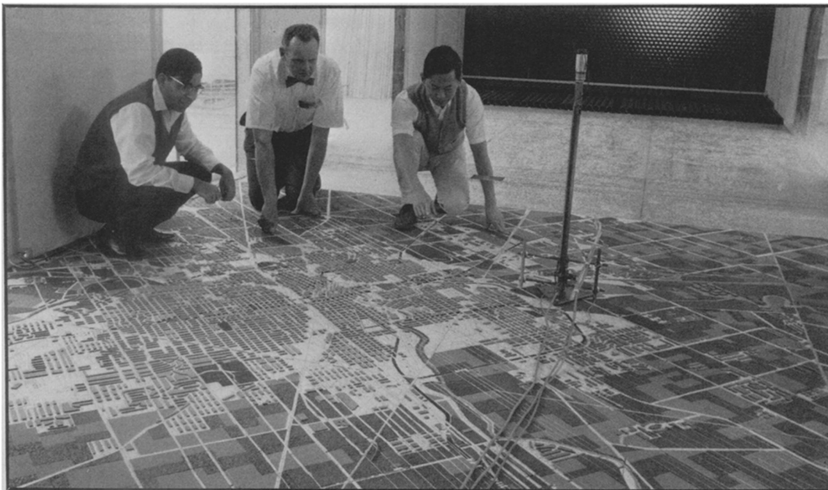
A 1:4,000 scale model of Fort Wayne, Ind., in CSU's environmental wind tunnel for pioneering study of heat-island effects on circulation of air pollutants. Heating elements provide surface-temperature distributions similar to those in city.
