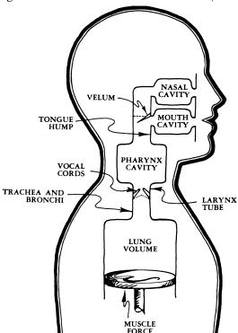
The human speech generation system consists of a hellows (the lungs) that pumps air past the vocal cords and through a series of resonating cavities (the pharynx, mouth, and nose). Nerve impulses regulate frequency and volume.
