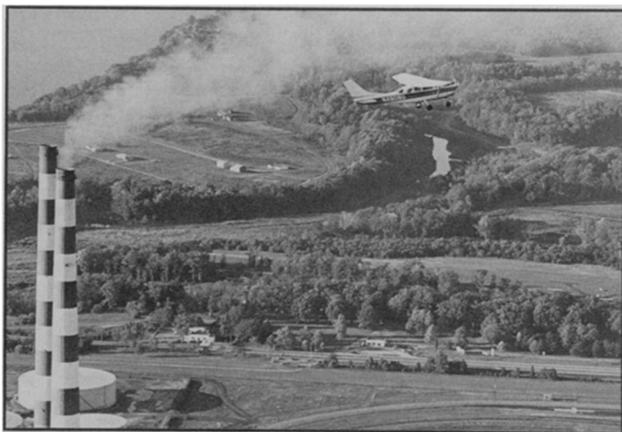
Chemists use specially equipped Cessna to sample pollutants emitted from Morgantown, Md., power plant.
