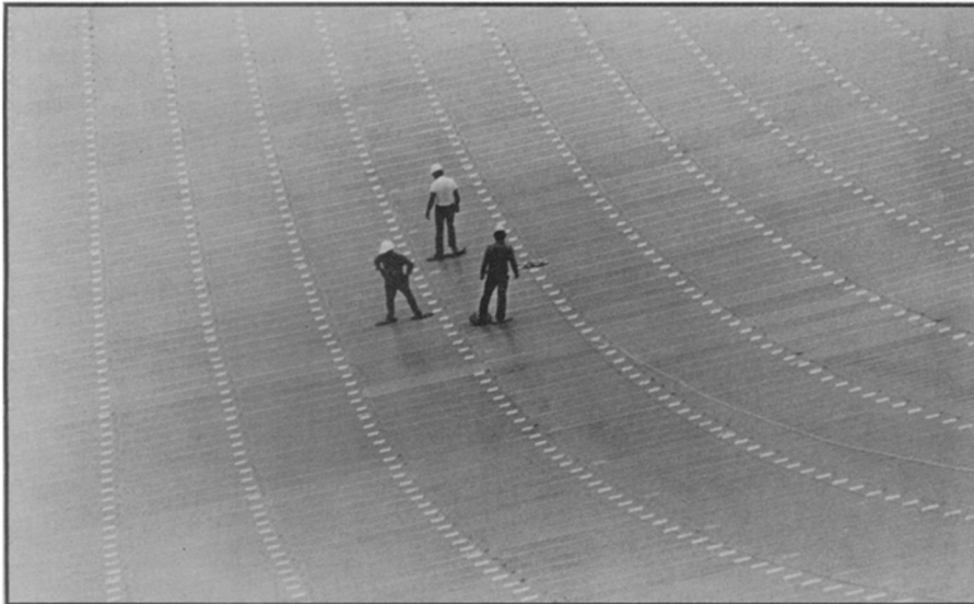
The white spots are laser targets for surveys that maintain the shape of the dish.
