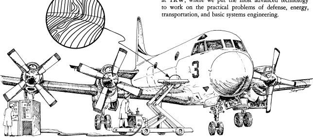
terferometry system, the equipment can be brought to the aircraft on a fork lift. Estimates show a time saving of as much as 50% with this kind of in situ inspection.
