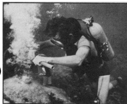
Hudson: Drilling coral cores.
