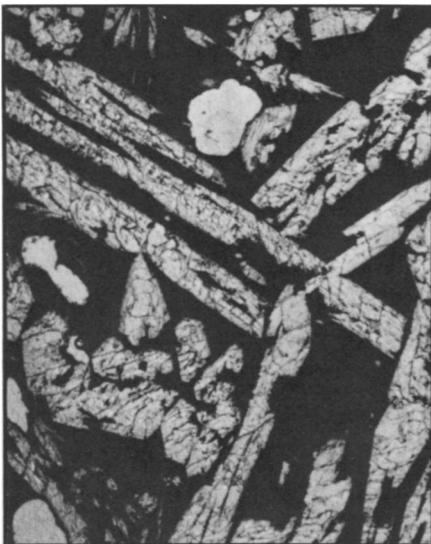
Faster cooling gave coarser texture to Apollo 15 sample of similar material.
