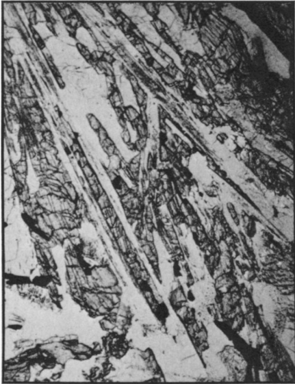
Apollo 12 basalt thin section shows mottled pyroxene, smooth plagioclase.
