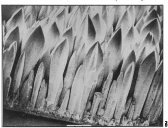
One of the keys to developing new energy technologies is materials research. IBM has developed a new type of light absorbing surface—shown here in electron micrograph—made of vapor-deposited tungsten. Some 96 percent of the light incident at the appropriate angle is absorbed, and the material can hold its heat at high operating temperatures (more than 900 degrees F.).
