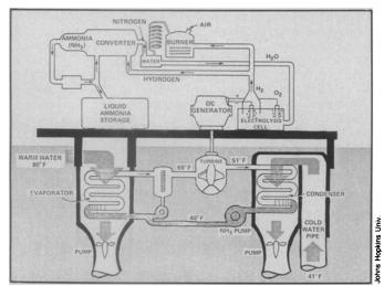
Ocean Thermal Energy Plant OTEP ships may help solve the food crisis as well as the energy crisis. By using the energy derived from ocean thermal gradients to make ammonia, at about one third the present cost, OTEP ships could help compensate for expected fertilizer and natural gas shortfalls a decade hence. Johns Hopkins University Applied Physics Laboratory is studying the possibilities.
