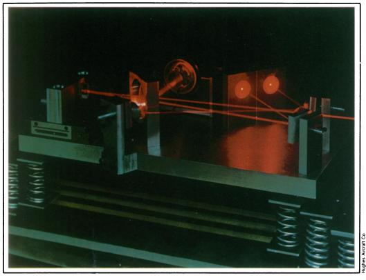
One form of possible gravity-wave detector uses laser beams to detect differential motions of test masses affected by the passage of the waves.
