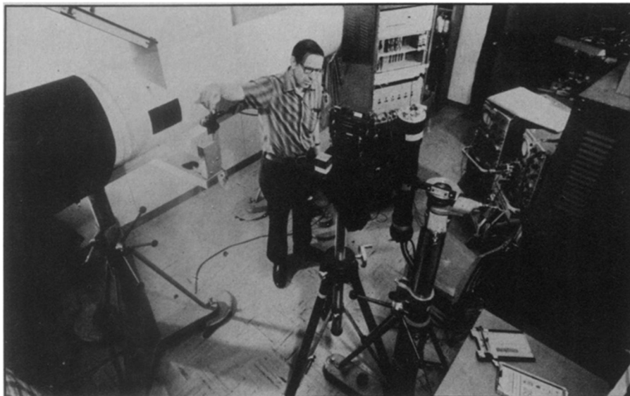
Robert G. Smits adjusts 12-inch telescope used at Berkeley for flexible-mirror tests.
