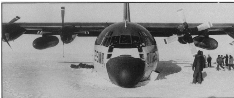
*Damaged during rescue mission, C-130 with collapsed nose gear nuzzles the snow.*
