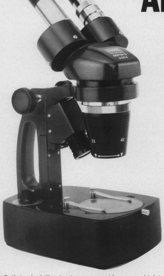
This stereo microscope was designed to serve college needs in viewing biological specimens, insects, ores, minerals and crystals, and the industrial market for scanning industrial parts and electronic components.
