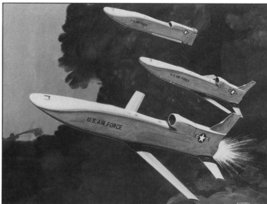
Air Force version of cruise missile spreads its wings and ignites its jet engine.
