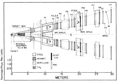
Paths of muon pairs are traced by arrays of detectors. Each arm contains an identical series.
