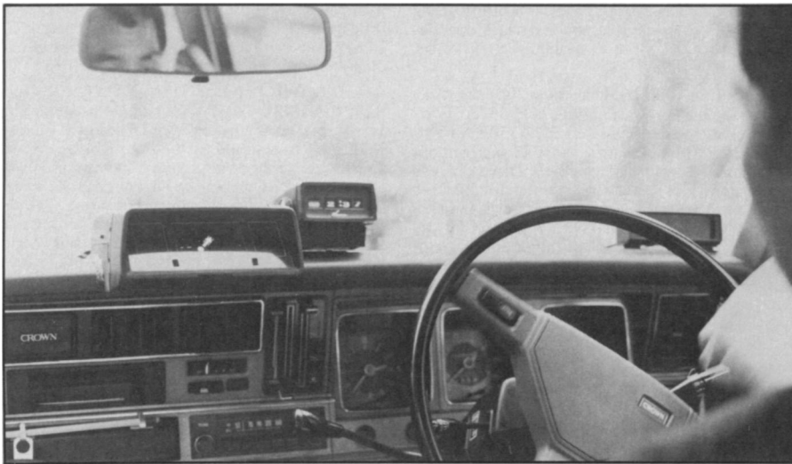
System installed. Route guidance display unit (below) shows approach to Y intersection.
