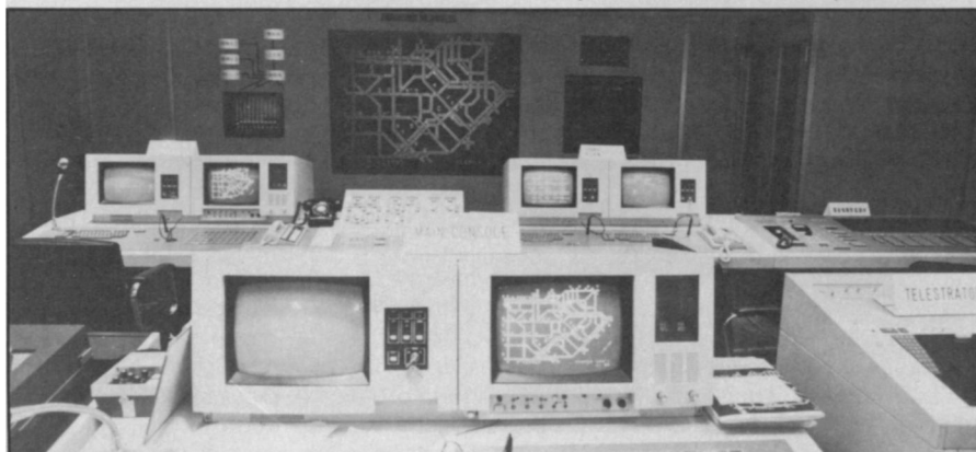
Central control room with traffic conditions and optimum routes on computer screen.
