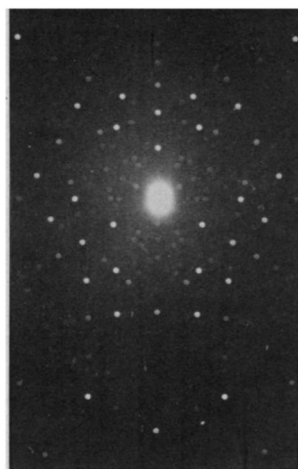
X-ray diffraction pattern produced by reflection from a nearly perfect gadolinium garnet wafer perpendicular to the X-ray beam (top). Enlargement of a single spot (elongated because of grazing incident reflection) from the image of a gadolinium garnet wafer on which an epitaxial film was grown and a metallurgical circuit pattern deposited (middle). Enlargement of a single spot from lithium fluoride crystal showing imperfections (bottom).
