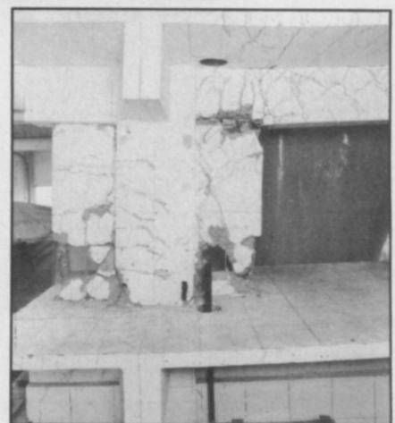
Model of ferro-concrete building elements undergoing static pressure (left). Detail of structural damage (right).
