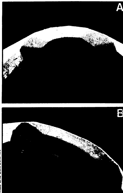
We have ways of making you yield. The flat face of a diamond anvil flowed into a permanent concave shape under 1.7 megabars pressure.
