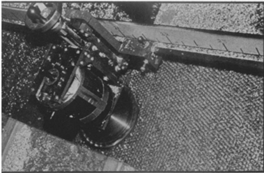
Honeycomb material is ground to mirror surface then coated with aluminum.
