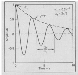
Data that represent the sum of a large number of damped sinusoids like the one immediately left can be analyzed by Prony's method. A computer at Livermore stores data representing individual vibration modes of a T-shaped metal plate and will add them at will (far left column). Still or moving pictures of the vibrations appear on the screen viewed by Darrel J. Lager (below).
