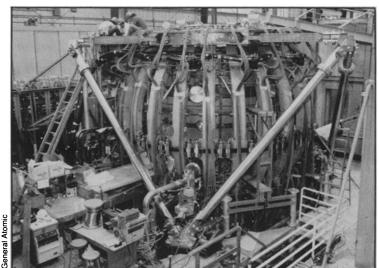
The vertical coils look a little bit like stays, and somewhere inside them is the chamber where Doublet III's plasma is expected to hold its hourglass figure as it slithers toward the day of breakeven.
