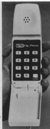
The Flip Phone flips open to reveal the keyboard and the privacy switch.
