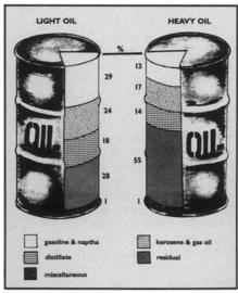
Fast traveling and gas guzzling add up to a high demand for the lighter fractions of the crude-oil barrel — gasoline, kerosene and naptha. Without upgrading, heavy crude produces mostly the thicker home-heating (distillate) and bunker (residual) oils.
