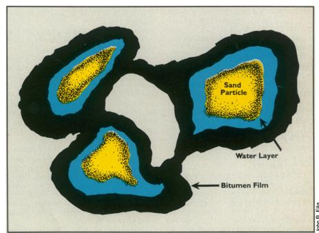
Oil does not occur in underground pools. Instead it surrounds individual grains of sand or coats the surfaces of porous rocks in a thin film. The goal is to bring up the oil with as little sand and rock as possible. Breaking the especially tough grip with which heavy oils cling to their host media generally requires heat and other means. Deposits where oils occur in a near-solid state — tar sands — offer the biggest challenge.
