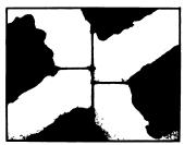
function as weakly superconducting links between larger, micrometer-sized regions of superconducting niobium thin films. Robert B. Laibowitz and colleagues at IBM have reliably produced and tested bridges as small as 40 nanometers (billionths of a meter) wide, 30 nm thick and 120 nm long.
