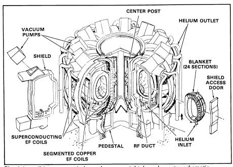
Plug it in; pull it out; screw it down. A commercial tokamak reactor schematic.
