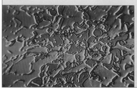
the technique to make GM 980X steel, comments, "I was working on another project using HSLA steel, when I noticed that if SAE 980X steel is heated above its eutectoid temperature (the temperature at which the crystalline structure of metal is transformed) for a few minutes, and cooled under controlled conditions, the steel developed significantly higher ductility and strain-hardening characteristics, with no reduction in tensile strength."
