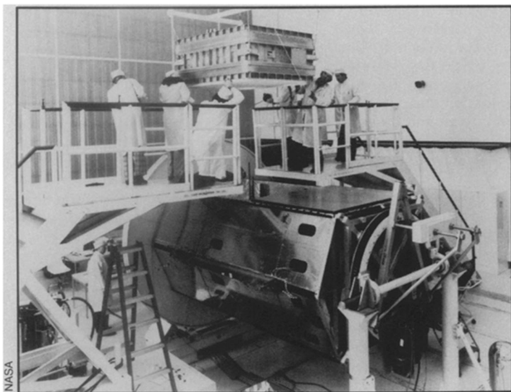
The French-Danish cosmic-ray isotopic composition experiment is placed aboard the HEAO-3 satellite.
