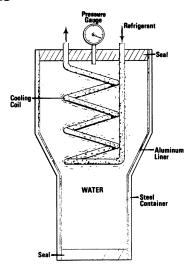
into intimate contact with the case. It involves cooling water against a loosely fitting aluminum liner. As some of the water freezes, pressure builds, sealing the aluminum firmly against the steel shell. The technique may be used to bind aluminum liners to steel or lead pipes that carry corrosive materials.
