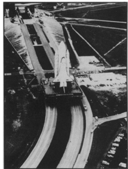
The space shuttle, being transported between its launch pad and assembly facility.
