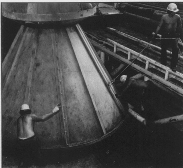
Re-entry cone is prepared for use on Leg 76. Cone, with three acoustic reflectors around its rim, remains on seafloor when pipe is withdrawn and allows the drill hole to be re-located and re-entered.
