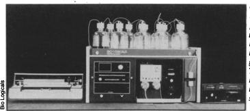
Gene machine automatically pumps chemicals through a column of particles that bind the growing chains. The operator need only specify the nucleic acid sequence.
