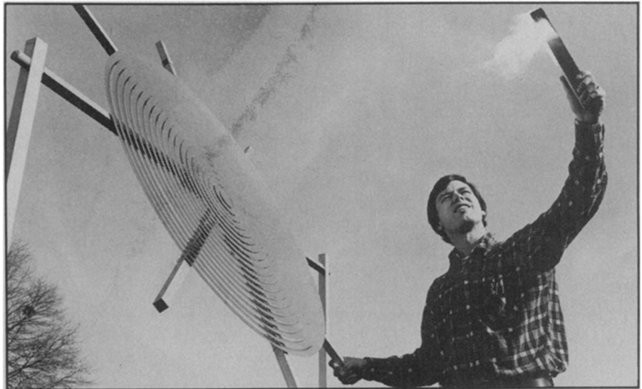
Anodized aluminum 500-sun concentrator ignites stick within two seconds.
