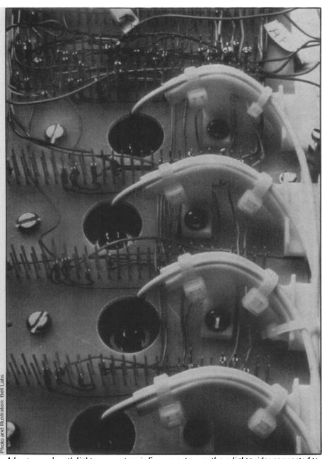
A long-wavelength lightwave system in Sacramento uses these lightguides connected to light-emitting diodes (LED's) instead of lasers. The LED's provide less light but last longer.
