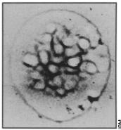
carbon-based photosensitive material called a resist. The scientists use X-rays to form a replica in the resist of the cell under study, and then they observe the resist in an electron microscope. The technique can resolve structures as little as 50 angstroms wide. Transmission electron microscopes can have higher resolution, but the samples must be thinly sliced and placed in a high vacuum. In addition, the X-rays may be used to distinguish different chemical elements in the cell.
