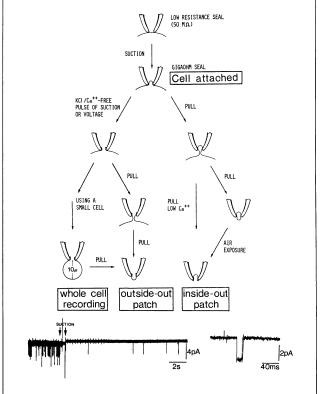
Sensitivity of signal is improved by slight suction (applied at center of top row of recording). Opening and closing of single channels can be detected (bottom row, larger scale than above).
