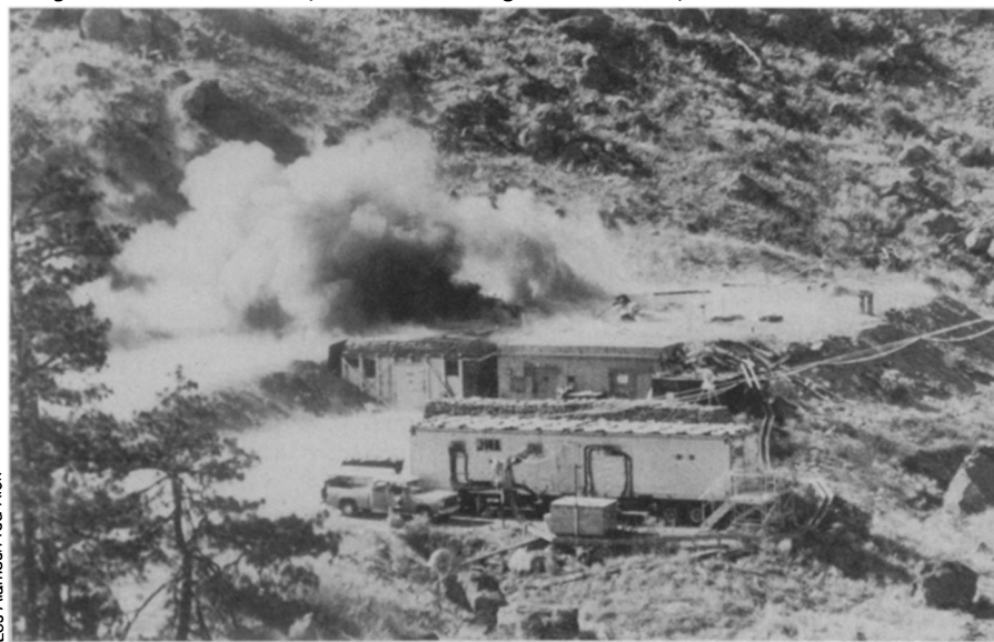
Railgun shot in Ancho Canyon: Another magnetic flux compressor raises the dust.
