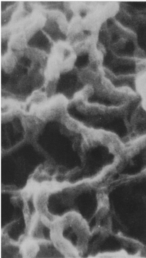
Scanning electron micrograph of polyacetylene. The upper photo shows the random fibrils (diameter \sim 200\text{\AA} ) that make up a shiny gray film when acetylene gas is catalyzed into an electrically conducting plastic. The lower photo shows the partial alignment from stretch orientation.
