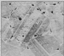
A scanning ion microscope photograph, top, of recrystallized, polished brass shows more detail than a comparable scanning electron micrograph because channeling of ions into properly oriented crystals creates greater contrast. In the ion photograph, the broad white band that bisects the large central crystallite contains dark details that may arise from defects or impurities within the crystal.
