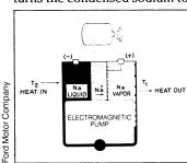
The device can use any source delivering heat at 700°C or more. Its efficiency, potentially in the range of 30 to 40 percent, is independent of the heat engine's size. A model designed for long-term testing has reached 19 percent efficiency at an output of 22 watts. The pump siphons off less than 0.1 percent of the energy out-
