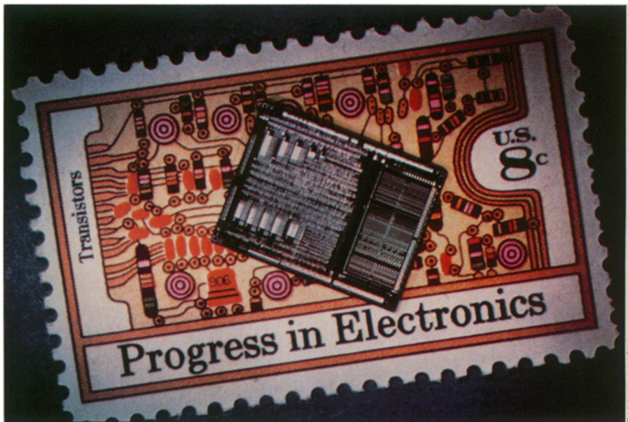
The invention of the transistor has led to integrated circuits such as the BELIMAC-32 microprocessor. The chip, only 1.5 centimeters square, has as much processing power as some minicomputers.
