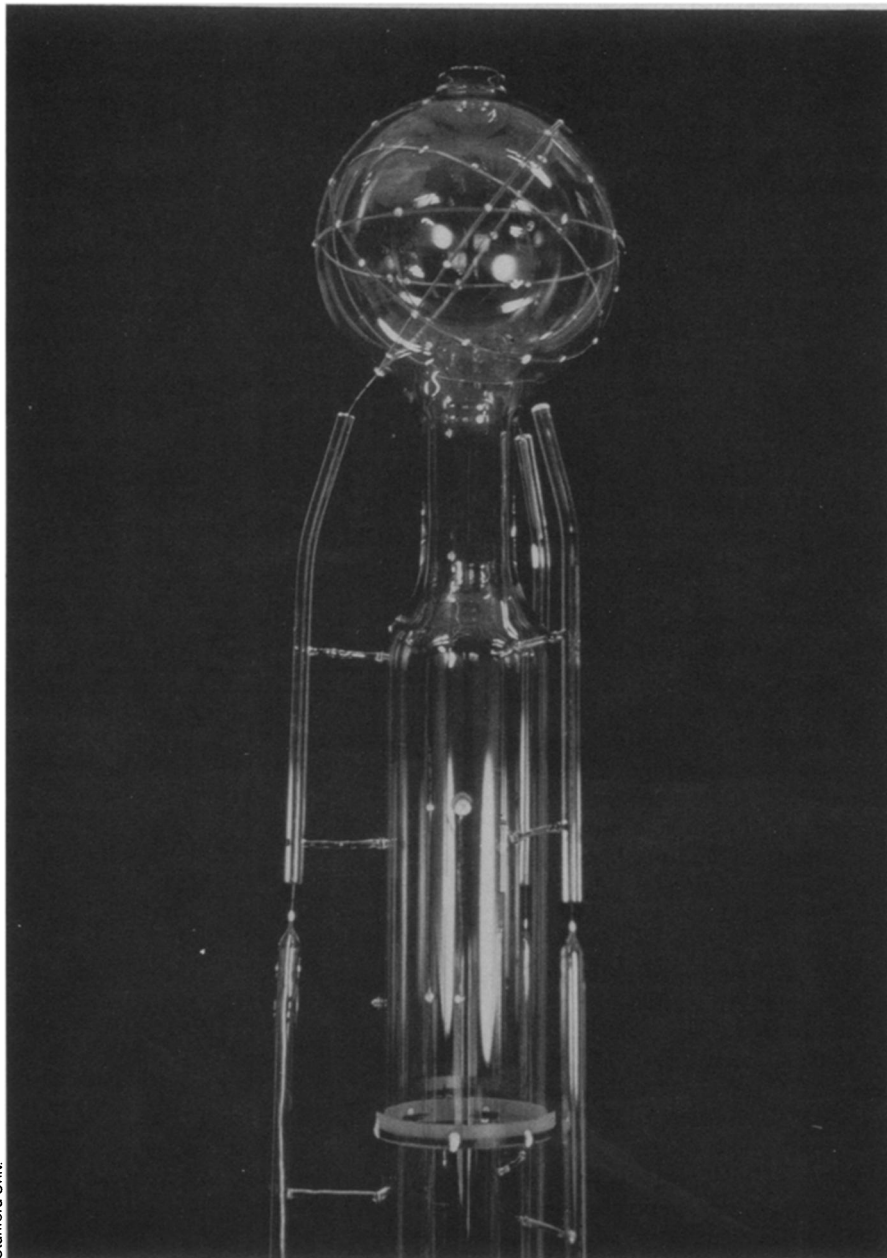
Blas Cabrera (standing, below) describes improvements to his monopole experiment. His new apparatus has detecting circuits with three perpendicular axes (above).
