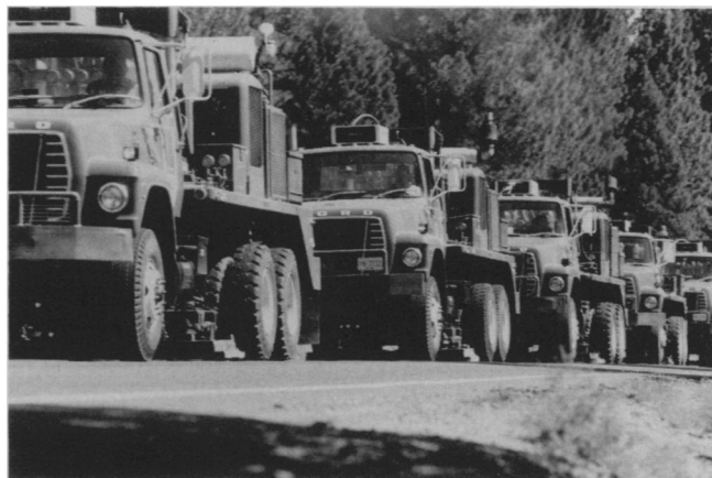
COCORP trucks inch along the nation's roads. They send vibrations through the earth and record the echoes as the seismic waves encounter layers in the crust.
