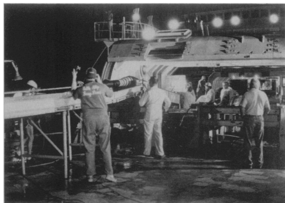
Cable for undersea use made of single-mode fibers was tested on the bottom of the North Atlantic. Here it is being payed off the stern of the cable ship Long Lines.
