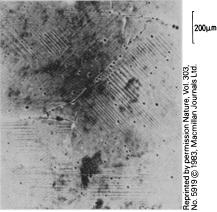
Although they can be detected in conventional unpolarized light, polarized light shows in greater contrast the crystal striations believed to be caused by surface tilts across magnetic domain walls.
