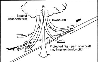
The downdraft spreads out as it approaches the ground. The plane, instead of flying a straight path to landing, first encounters a headwind, which lifts its nose, and then a strong tailwind, which forces the nose down. At low altitudes the pilot sometimes cannot compensate for the wind changes, and the plane crashes.
