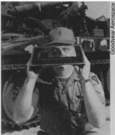
New vision blocks being developed for the Army at Goodyear Aerospace Corp. in Litchfield Park, Ariz., are now able to provide protection that in some cases actually matches that of surrounding metal armor. Experimental test versions are from 4-inches to 8-inches thick, weigh 16 to 23 pounds, and provide a 12-inch by 4-inch viewing window.
