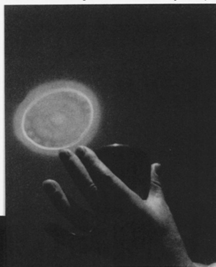
When a makyo reflects light, the design inscribed on its back shows up in the reflection (above). Typical designs include figures of Buddha and famous quotations (left).
