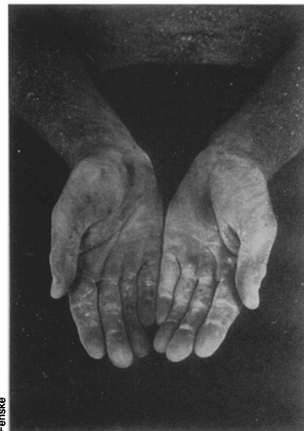
Under ultraviolet illumination, bright spots mark where the toxic pesticide has penetrated a worker's protective clothing.
