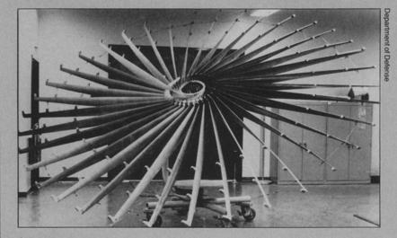
Should intercontinental ballistic missiles (ICBMs) begin to rain, here's what the Defense Department might put up — a pinwheel-shaped structure that unfurls from about the neck of an intercepting missile just before the two projectiles collide. Its roughly 7-foot metal ribs, shaped like framing struts of an umbrella, are seeded with steel weights. This
