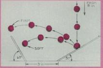
metal core to move through the magnetic coil, generating a voltage, Davis explains. Soft berries are identified by the time it takes them to displace the speaker coil; the voltage waveform they generate takes longer to achieve its peak amplitude.
